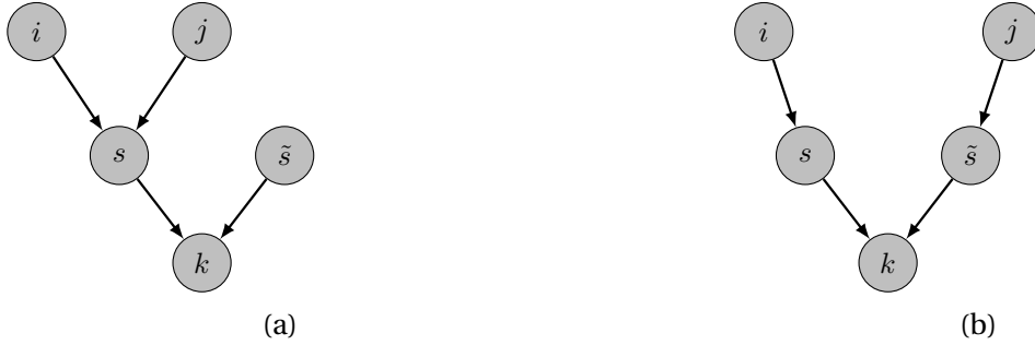
Figure 1. Two simple production networks where each vertex corresponds to an industry, with a directed edge present from one vertex to another if the former is an input-supplier to the latter. Industry k is downstream to industries i and j in either case. In panel (a) the input paths from i and j to k overlap; in panel (b) they do not.
